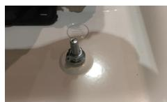
Insert the eyelet cable to the Earthing screw and fasten the whole using another washer and nut.
