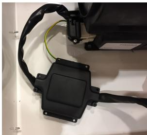
Insert the earthing screw from the outside inwards, fastening washer and screw as indicated.
